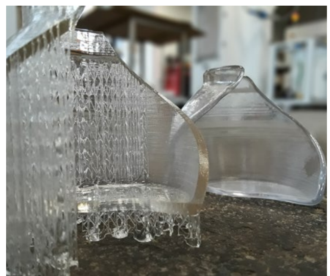
3D printed SLA parts, before and after post-processing. Image: PostProcess Technologies
